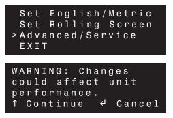
The warning screen will show, press the UP ( $\blacktriangle$ ) button to continue. To return to the Primary Menu, move the cursor (>) to EXIT and press the MENU/EXIT ( $\leftarrow$ ) button.
