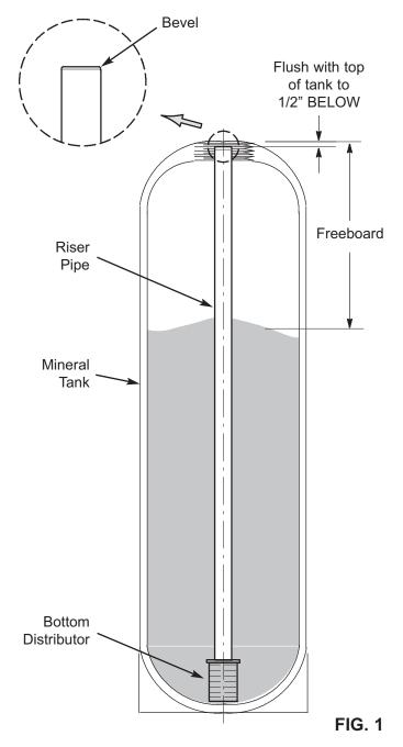
**Note:** Resin tank height can vary somewhat within manufacturing tolerance. So to be sure the bottom distributor riser pipe has proper clearance with inside valve porting, check for the correct length, as shown above. Cut the riser if needed to adjust the length. Be sure to remove burrs and sharp edges.
