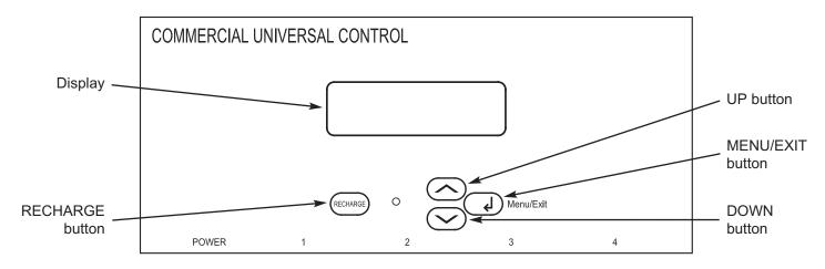
The CUC2 is a menu-driven electronic controller with a dot matrix display. The UP ( $\checkmark$ ) and DOWN ( $\checkmark$ ) buttons move the cursor (>) up and down the menu choices. The MENU/EXIT ( $\leftarrow$ ) button enters the value selected and returns the display back a level. The controller will return to the normal operating screen after 4 minutes, if left in a menu and no selection has been made.
