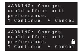
The warning screen will show. Press the RECHARGE button to toggle the padlock icon. Press the MENU/EXIT (↔) button to select and return to the Primary Menu.
