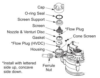
IMPORTANT: Be sure small hole in the gasket is centered directly over the small hole in the nozzle & venturi housing. Be sure the numbers are facing up.
