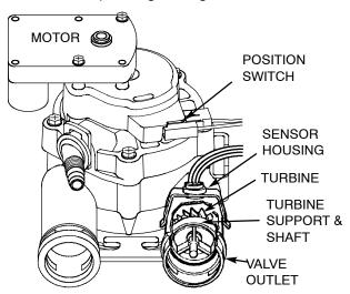
If you don't get a reading in the display, with faucet open, pull the sensor from the valve outlet port. Pass a small magnet back and forth in front of the sensor. You should get a reading in the display. If you get a reading, unhook the in and out plumbing and check the turbine for binding.
