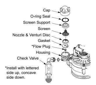
IMPORTANT: Be sure small hole in the gasket is centered directly over the small hole in the nozzle & venturi housing. Be sure the numbers are facing up
