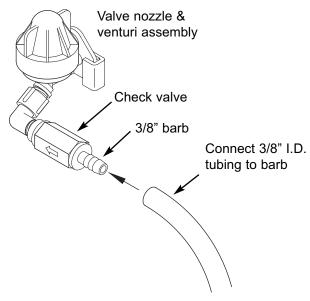
Place other end of tube in hydrogen peroxide solution
